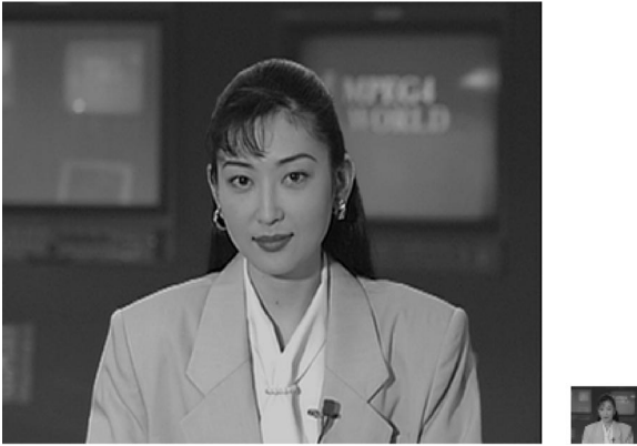
Fig. 11. A full image (352 × 288 pixels) and its DC image (44 × 36 pixels).
