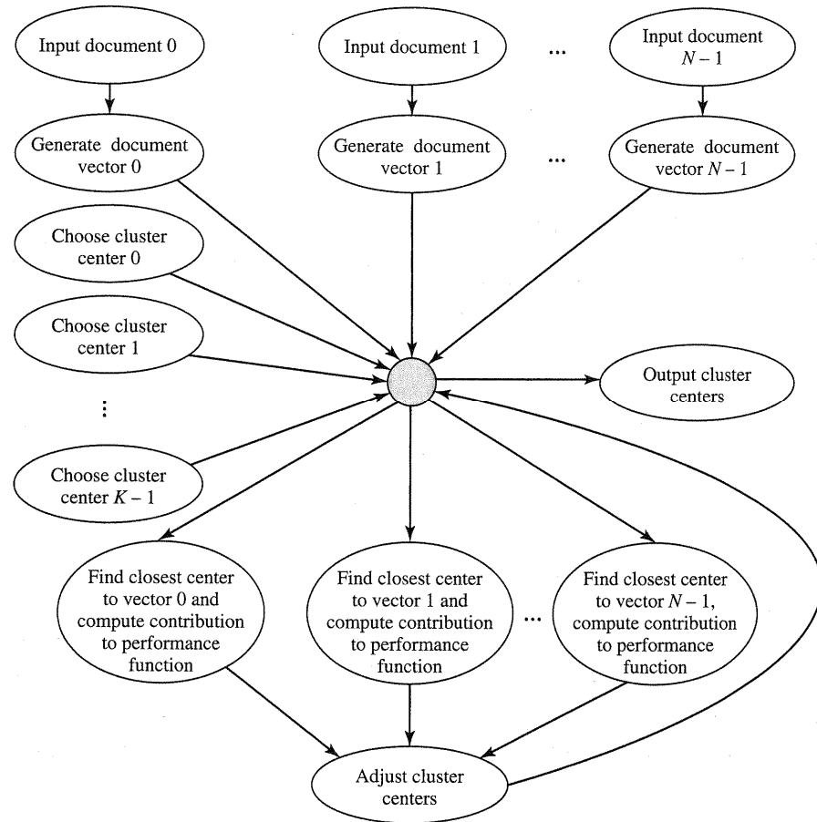
Figure 1.9 Dependence diagram for the document clustering algorithm. The small, unlabeled vertex in the middle is a “null task” containing no operations. Its purpose is to reduce the number of directed edges and make the diagram easier to read.
