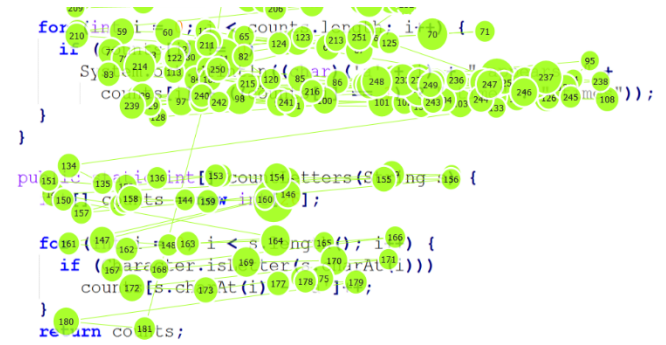
Fig. 1. Gaze plot of a developer's fixations on code.
