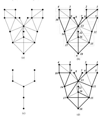
**Fig. 1.** (a) A chordal graph G. (b) A BFS-ordering  $\sigma$ , BFS-tree T associated with  $\sigma$  and a layering of G. (c) The tree  $\Gamma$  of G associated with that layering. (d) Additive 4-spanner (actually, additive 3-spanner) H of G constructed by PROCEDURE 1 (5 edges are added to the BFS-tree T).
