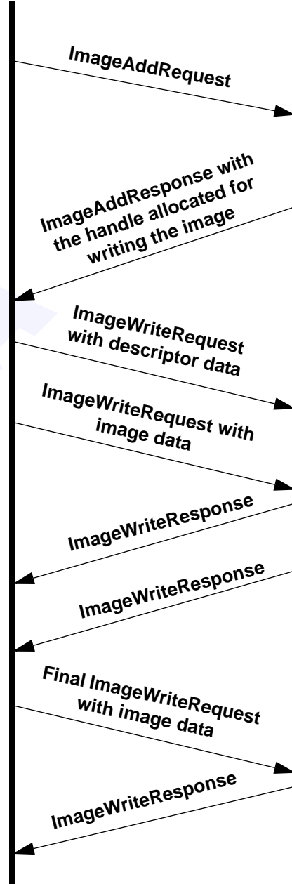
Figure 287 Ladder Diagram of Image Write operation
