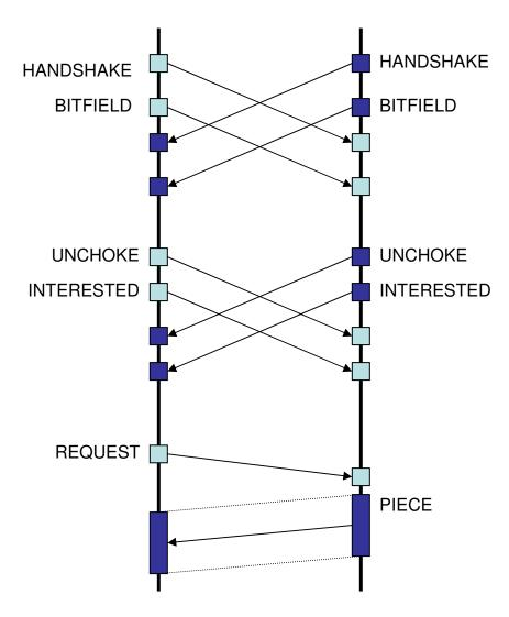
Fig-3 Typical message sequence between two TiniTorrents exchange slaves.
