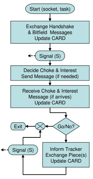
Fig-2 Piece Exchange Slave of TiniTorrent.
