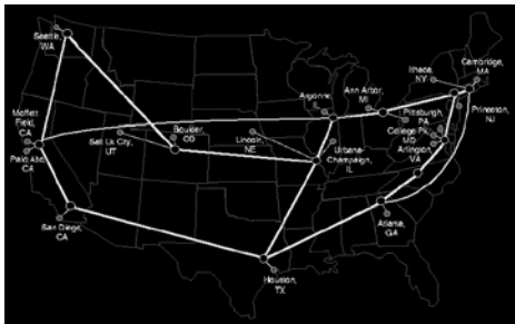
The Wide Area Network that formed the backbone of the Internet before 1992. Funding came from NSF, IBM, MCI, and MERIT
