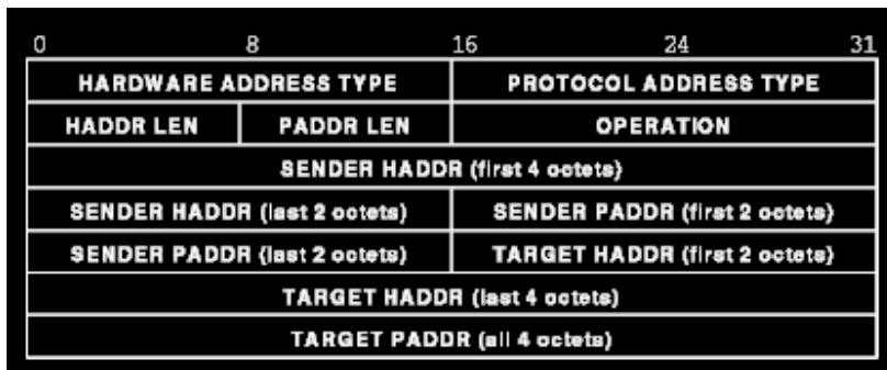
IP to Ethernet ARP message format
