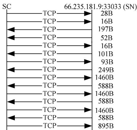
**Figure 5. Message flow for first login after installation for a SC behind a firewall, which blocks UDP packets. ‘B’ stands for bytes and ‘N’ stands for node. SYN and ACK packets are shown to indicate who initiated TCP connection. Message flows are not strictly according to time. Messages have been grouped together to provide a better picture. Message size corresponds to size of TCP or UDP payload. Not all messages are shown in the message flow.**
