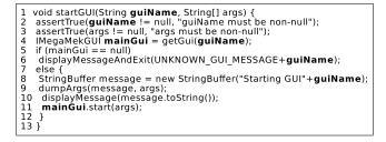
Figure 4. Eliminating a use of the formal parameter (Line 6) in an infrequently executed block (Line 5).
