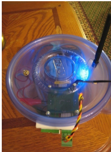
Figure 2: Packaging of Oxybuoy electronics for the DO lab experiment.
