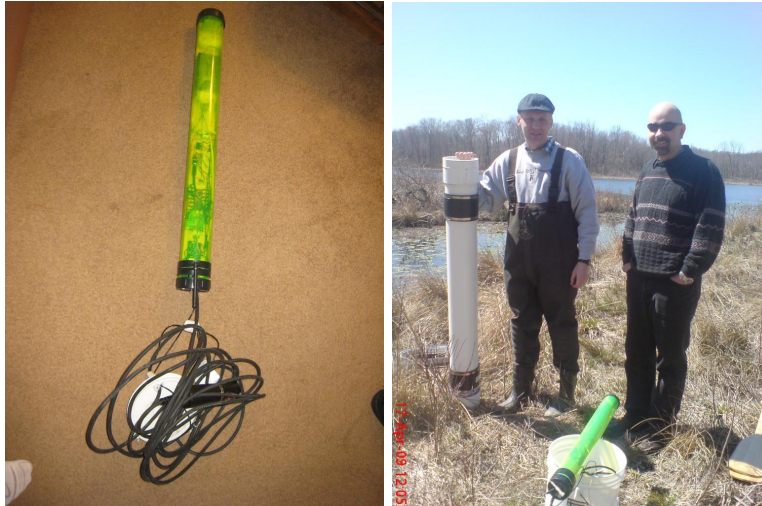
(a) Electronics packaging of Oxybuoy. (b) Oxybuoy ready for assembly before deployment.
