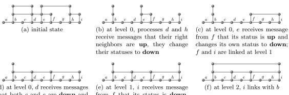
(d) at level 0, d receives messages that both c and e are **down** and changes its status to **up**, links with neighbors at level 1
