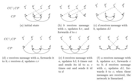
Fig. 2. Example computation of l-Corona. To simplify the picture each process is represented by two nodes. The primed nodes are the process' incoming channel. Solid lines denote identifiers stored in l and r of each process. Dashed lines are identifiers in the incoming channel.
