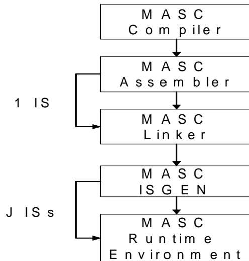
**Figure 2: MASC phases of compilation including the ISGEN phase.**
