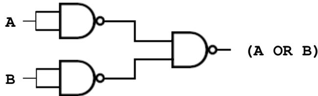
The input A is fed as the two inputs to the first NAND gate and similarly B to the second NAND gate. The third NAND gate produces the correct output for A OR B. It may be interesting for the reader to verify that this implementation works for all possible values of A and B.
