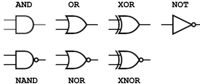
More complicated digital circuits are built by wiring together logic gates. Pulse signals, typically produced by a crystal oscillator, provide a processing rhythm. The next processing step won't start until a new clock pulse arrives. The pulse interval is needed for all digital signal transitions to complete and the circuit components to settle into their new states. Typical clock rates for modern CPUs are in the GHz range.
