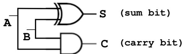
Here we used an XOR gate to produce the sum bit and an AND gate to compute the carry bit. Table 2 lists the input and output values for the half adder. The half adder shows how logic gates are used to add two bits.
