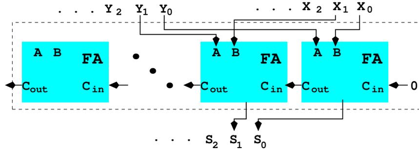
Because the carry bit may need to propagate from the rightmost adder all the way to the leftmost, a delay proportional to  $n$  is needed until the last output bit settles down. Such an adder is known as a *ripple adder*. More complicated adders can reduce the delay and make binary addition faster, especially if addition is performed as a subprocess of multiplication.
