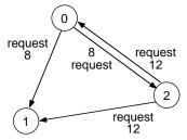
■ Threads 1 and 2 reply, thread 0 defers and enters the CS since its request was first:
