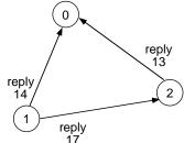
■ After leaving the CS, thread 0 replies to thread 2, which enters the CS
