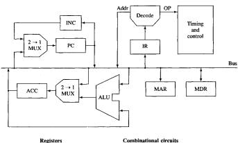
ACC (accumulator) IR (instruction register) MAR (memory address register) MDR (memory data register) PC (program counter)
