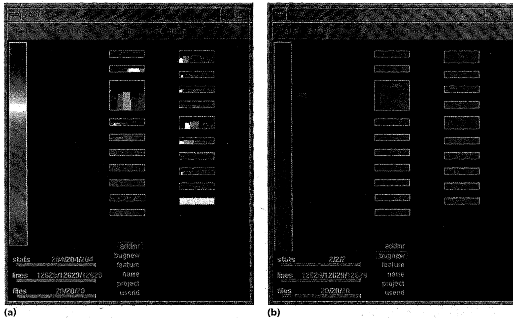
Figure 4. Summary representation. Each file is represented as a colored rectangle with a small plot inside. For each file, (a) shows the code age (blue represents the old code and red the new), while (b) shows the amount of bug-fixing code relative to new feature development.
