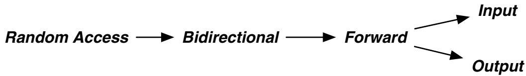
Figure 2. Refinement relationships among the STL iterator concepts, where an edge A \rightarrow B is read as “ A refines B .”
